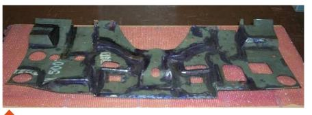
Picture above shows a traditionally manufactured firewall in multiple, overlapping and welded plates.
